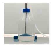
3. Place the metal nozzle of the dispensing line inside of the supplied bottle.
