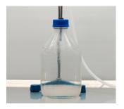
3. Place the metal nozzle of the dispensing line inside of the supplied bottle.
