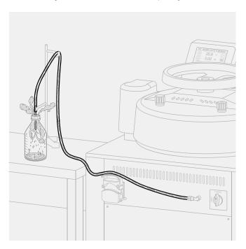
beginning the sterilization phase is always activated automatically. Therefore, the metal nozzle must be placed inside the bottle provided with the media preparator to avoid possible burns and to collect the condensed steam that is expelled during this procedure. After completing this step, when starting the dispensing phase, the metal nozzle should be removed from the bottle. It is very important not to use any other bottle to collect this steam than the one supplied by RAYPA.
