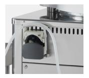
${\bf 2.}$  Check that the dispensing line is not pinched by the peristaltic pump or the external dosing station.
