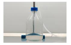
3. Place the metal nozzle of the dispensing line inside the bottle supplied with the media preparator.
