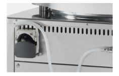
2. Check that the dispensing line is not pinched by the peristaltic pump or the external dosing station.
