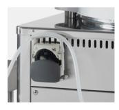
2. Check that the dispensing line is not pinched by the peristaltic pump or the external dosing station.
