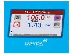
Digital microprocessor with a 5" TFT touchscreen for an easy programming and parameters selection.
