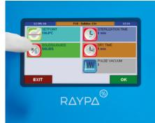
Several process parameters are shown on the screen such as current temperature, current pressure, both in numbers and in graphs, including water status or heating status.
