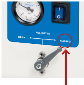
THE VALVE (9) MUST BE IN THE "CLOSED" POSITION WHEN FILLING THE INDEPENDENT WATER TANK AND DURING REGULAR OPERATION OF THE AUTOCLAVE.
