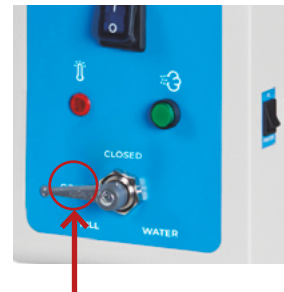
THE VALVE (12) MUST BE IN THE "OPEN" POSITION TO DISPENSE WATER INTO THE STERILIZATION CHAMBER.
