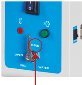
THE VALVE (12) MUST BE IN THE "CLOSED" POSITION WHEN FILLING THE INDEPENDENT WATER TANK AND DURING REGULAR OPERATION OF THE AUTOCLAVE.
