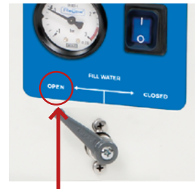
THE VALVE (9) MUST BE IN THE "OPEN" POSITION TO DISPENSE WATER INTO THE STERILIZATION CHAMBER.
