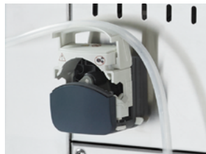
2. Check that the dispensing line is not pinched by the peristaltic pump or the external dosing station.
