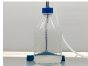
3. Place the metal nozzle of the dispensing line inside of the supplied bottle.
